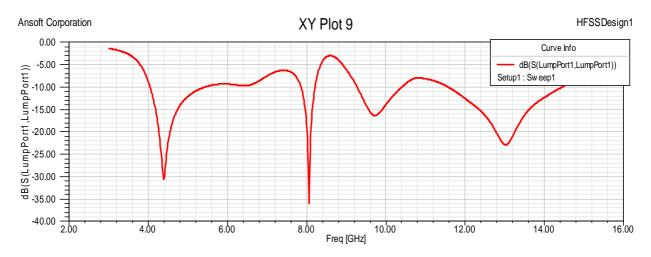
Fig 2: Return loss v/s frequency curve for varying length of ground plane
