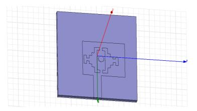
Figure 1: Design of Partial slot T-shape Patch Microstrip Antenna
