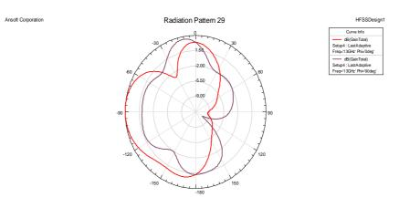
Figure 6: 2D E-plane Radiation Pattern at 13 GHz
