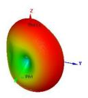
Figure 8: 3D Radiation Pattern at 13 GHz
