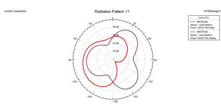
Figure 5: 2D E-plane Radiation Pattern at 7.2 GHz
